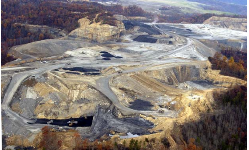
Mountaintop Removal Mining in Perry County, KY (Photo courtesy of the Mountaintop Removal Road Show):
